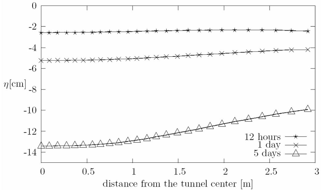
Figure 6. Surface settlement with time (case of 10 drains and  $K=1.E-08m/s$ )
