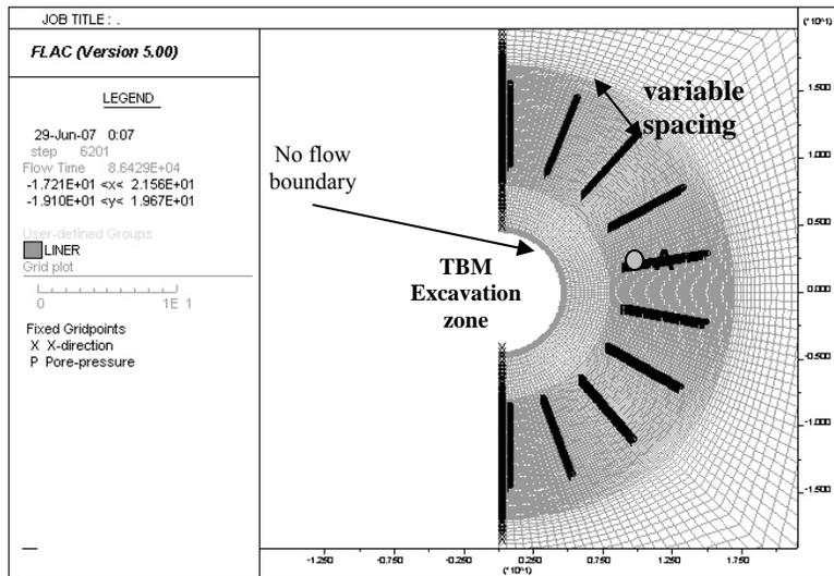
Figure 3. Scheme of the simulation - detail of the FLAC mesh close to the pre-excavated tunnel (case drains only)
