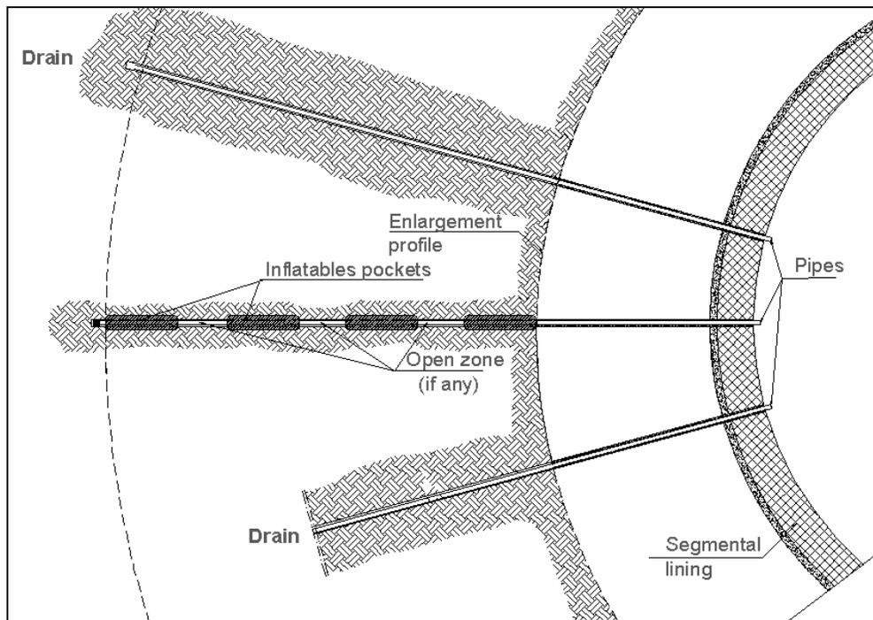
Figure 1. Combination of radial drainage and volume-controlled grouting
