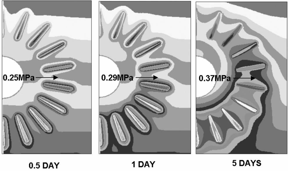
Figure 4. Pattern of the isotropic effective stress  $\sigma'_0$  close to the crown of 10 drains for  $K=1.E-08m/s$
