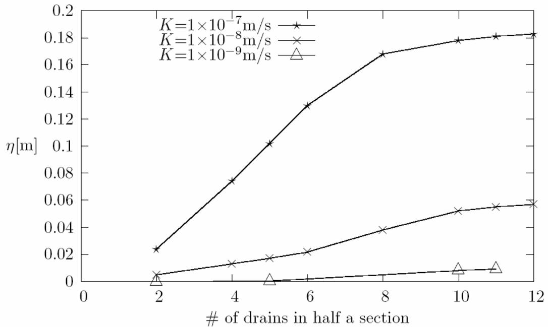
Figure 7. Maximum surface settlement at 1 day plotted against the number of drains and per each selected K value
