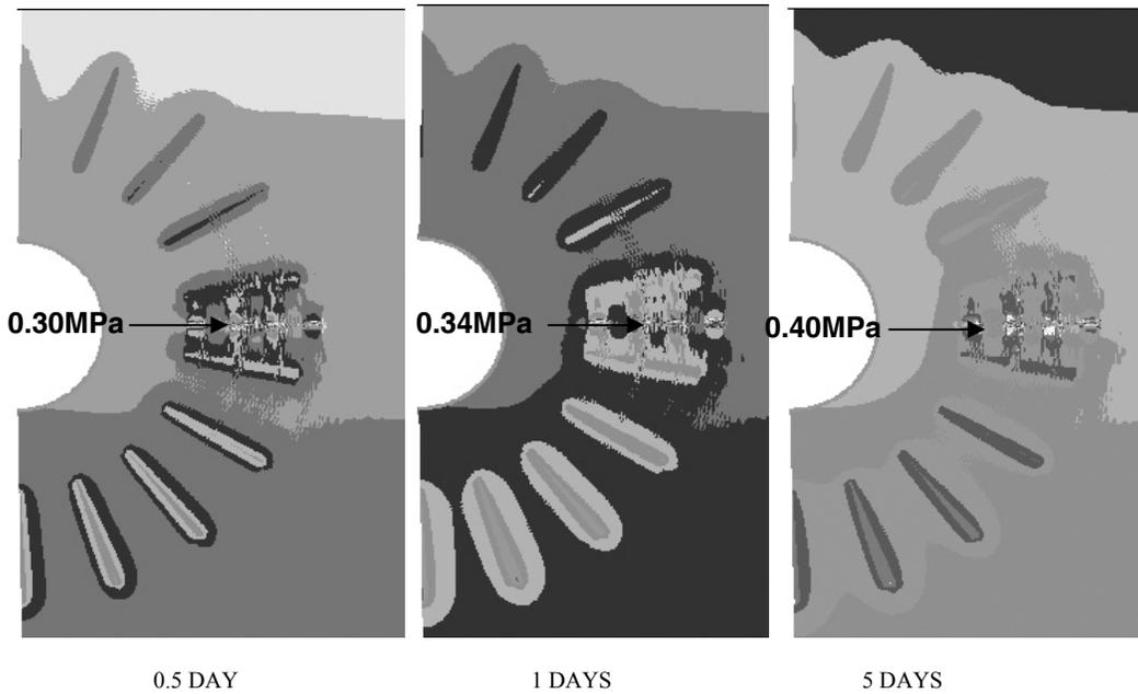
Figure 9. Pattern of the isotropic effective stress  $\sigma_0'$  close to the crown of drains for  $K=1.E-08m/s$ , 10 drains and volume-controlled grouting
