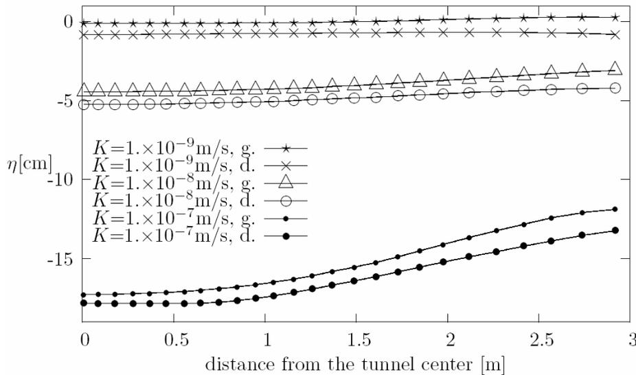
Figure 10. Surface settlements for each selected  $K$ ; comparison between drains-only (d.) and drains+grouting (g.) cases (10 drains) after 1 day
