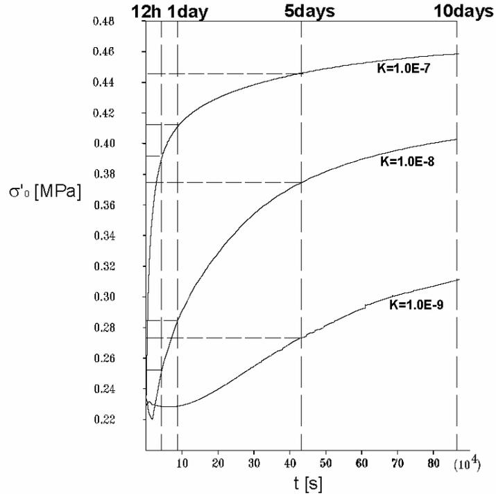
Figure 5. Evolution of  $\sigma'_0$  with time at node A for each selected K value (case 10 drains)
