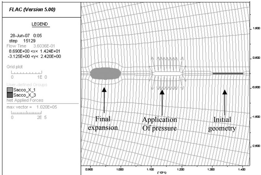
Figure 8a. Expansion of the inflatable pockets (application of pressure)
