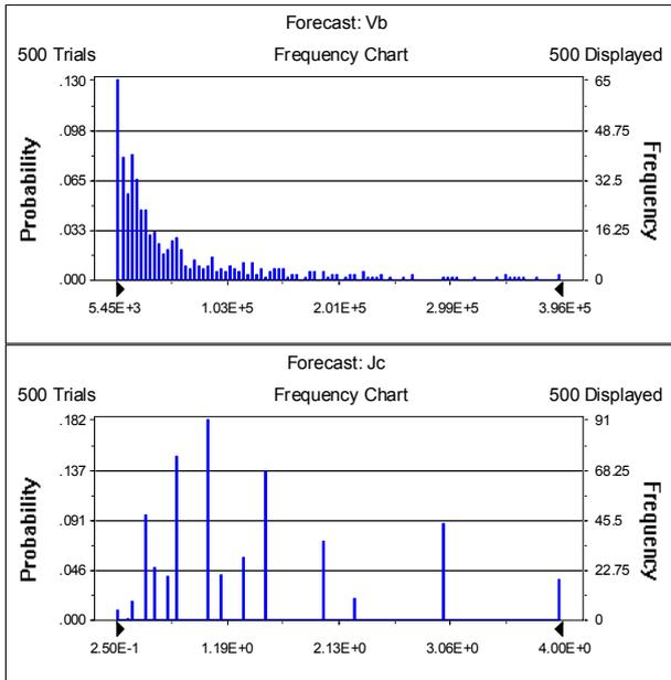
Fig. 4.1 (b) : Example of probabilistic quantitative assessment of GSI. Calculated parameters ( $V_b, J_c$ ). The derived GSI distributions for both the applied methods are reported in Fig. 4.2 (a,b) and compared in Fig.4.4 and Tab.4.1.
