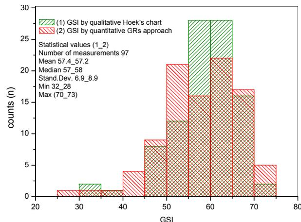
Fig. 3.6 (b): Comparison of the histograms and statistical values of the GSI for the n. 97 geostructural surveys realized.
