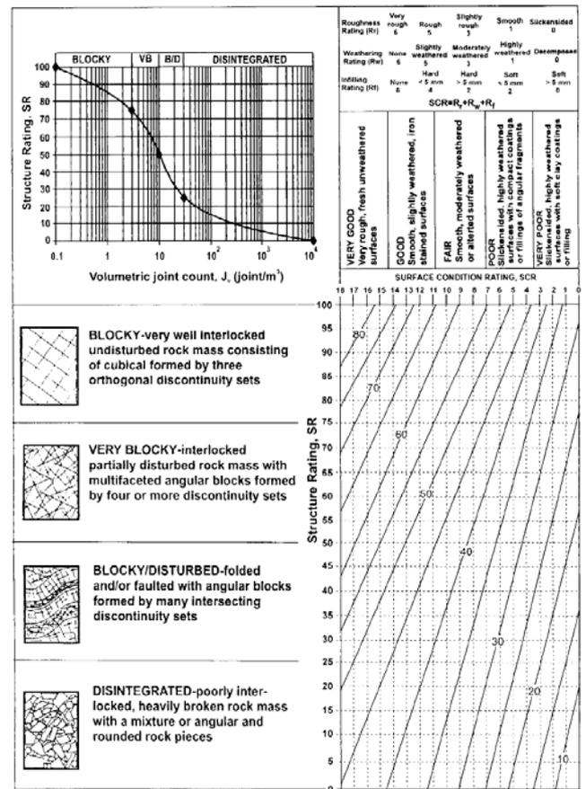
Fig.2.1: Modified Hoek's chart for the determination of the GSI proposed by Sonmez and Ulusay [31].
