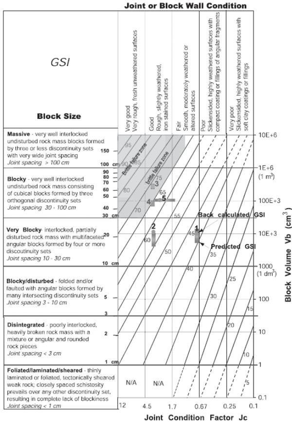
Fig. 2.2 Hoek's chart (1999) for the determination of the GSI modified by Cai et al. [10].
