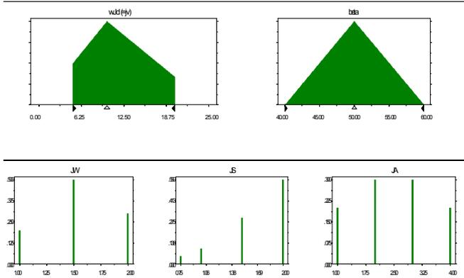
Fig. 4.1 (a): Example of probabilistic, quantitative assessment of GSI. Input parameters (from left to right)→ above:  $wJd(\approx \beta)$ ,  $\beta$ ; below:  $jW$ ,  $jS$  and  $jA$
