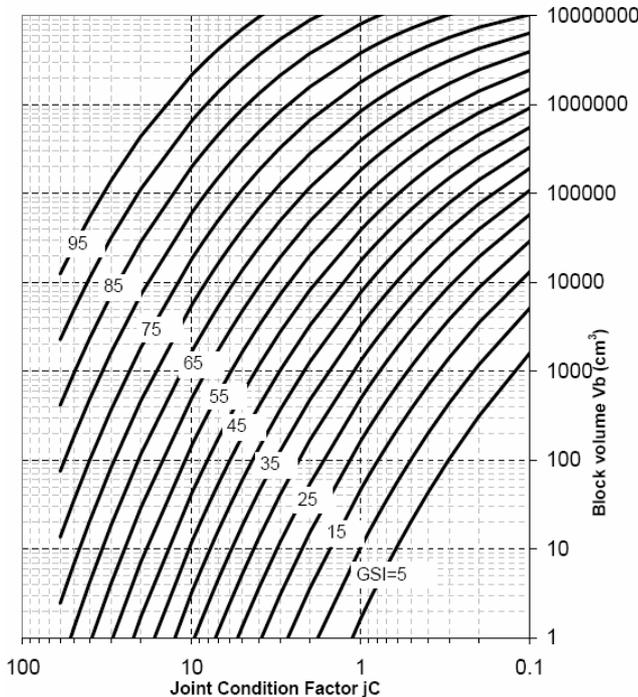
Fig. 3.2: New proposed diagram for the assessment of GSI by means of the Rmi parameters  $jC$  (see in Appendix) and  $V_b$ .
