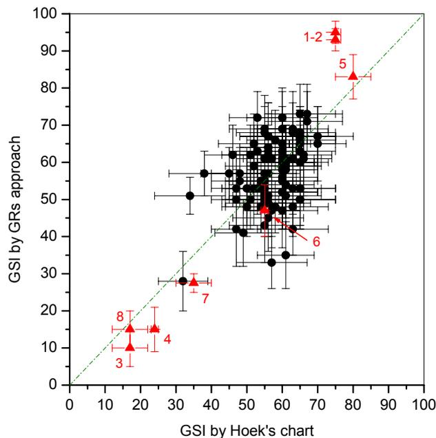
Fig. 3.6: Comparison between the GSI values in Figs. 3.5 (triangular symbols, references in Bibliography), as well as between the results of n.97 geostructural surveys (black circles) in the Alpine structural domain. For the new quantitative approach ("GRs"), the probabilistic method has been implemented, as further described in the Section 4, and the error bars in the figure correspond to two times the standard deviation.
