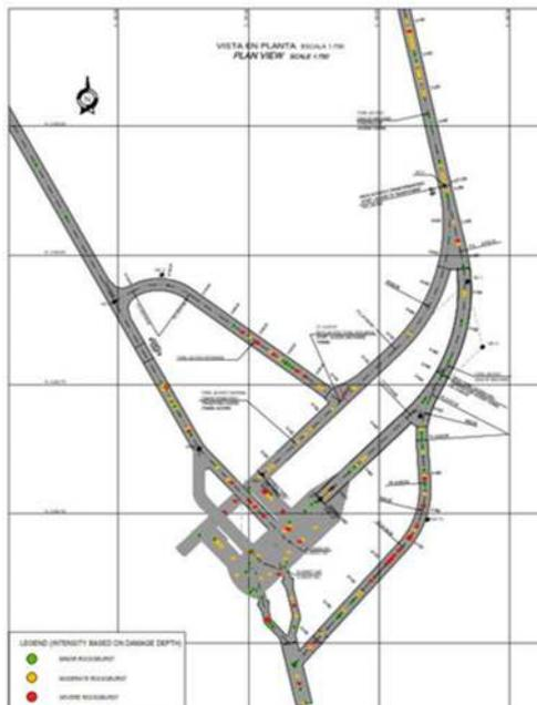
Figure 13. Rockburst locations and damage severity in the zone of the Powerhouse
