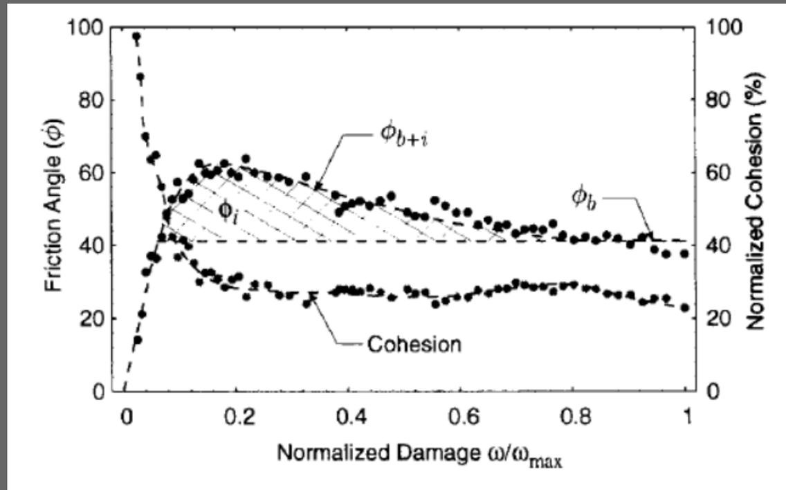
In brittle rock the mobilization of the cohesive and frictional component is strain dependent. Cohesion mobilizes before than friction angle [ $\phi_b$  and  $\phi_i$  are residual and interlocking (dilation) component] → "m=0 approach"
