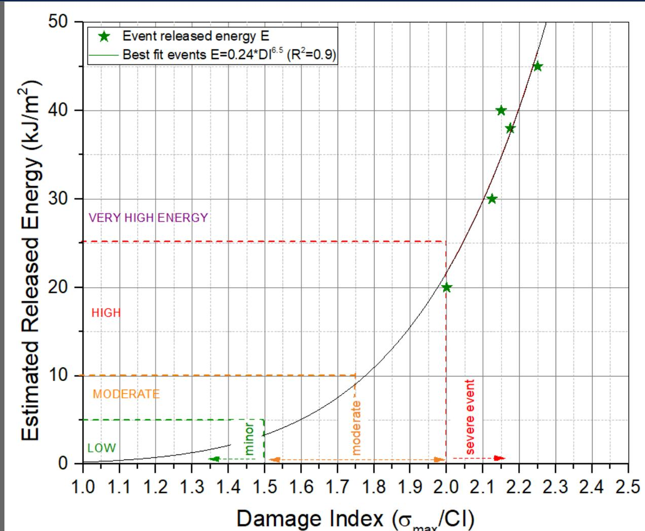
**Example of relationship between Damage Index and estimated Released Energy of severe rkb events in Andesitic rocks**
