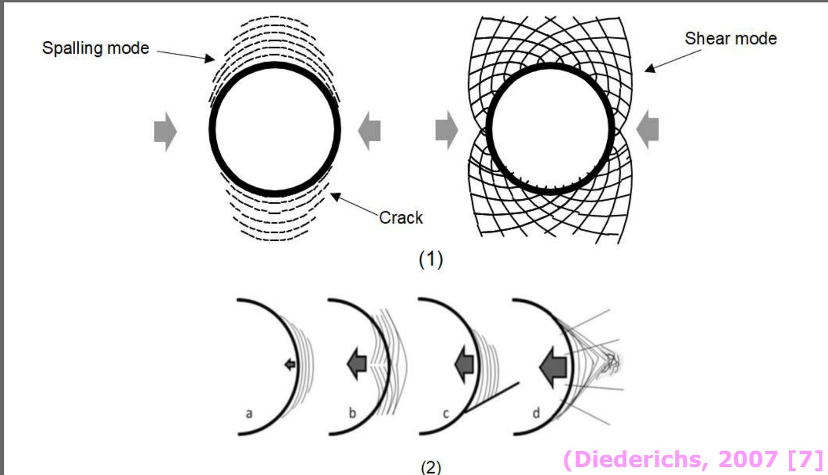
**1) Creation of boundary parallel spalling fractures compared to the progressive shearing assuming in plasticity; (2) Transition from non-violent spalling (a) to bursting through buckling (b), interaction with structure (c) and dilational yield (d)**
