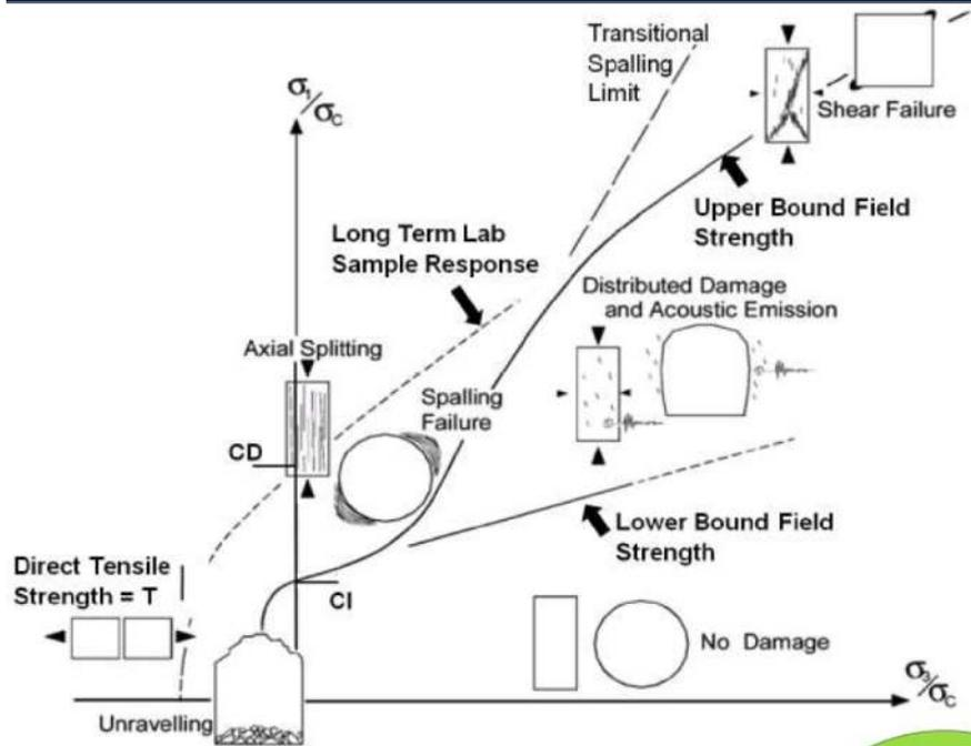
The composite strength envelope illustrating in principal stress space the zones of behaviour as bounded by the damage initiation threshold, the upper bound shear threshold (damage interaction), and the transitional spalling limit
