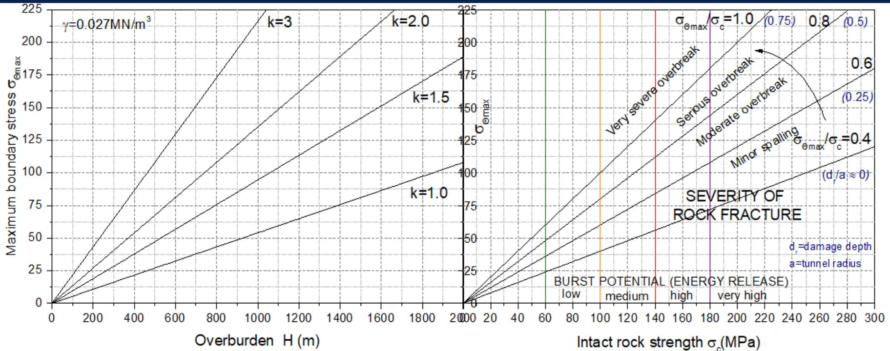
Chart for assessment of the severity of brittle rock failure [27]
