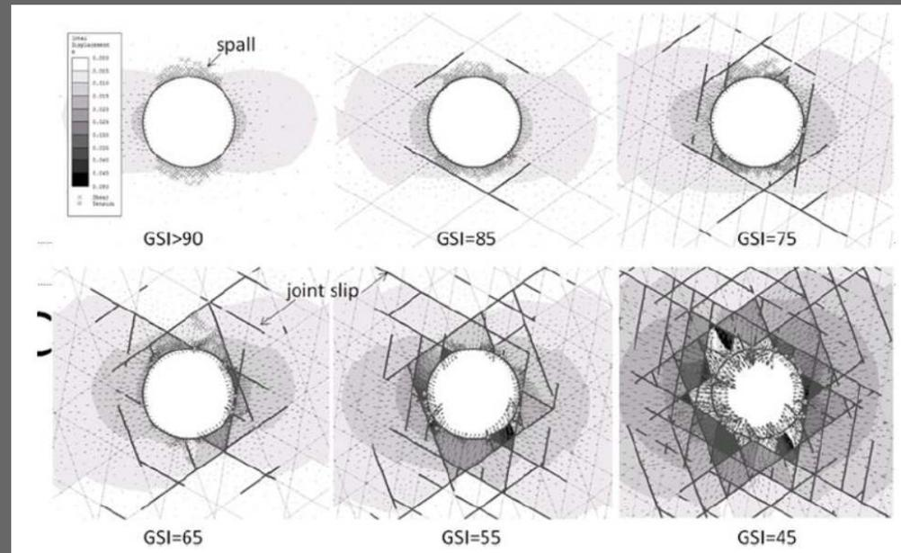
**Guidelines for analysing rock failure as shearing or spalling based on GSI and the ratio of compressive to tensile strength (→strainburst susceptibility)**
