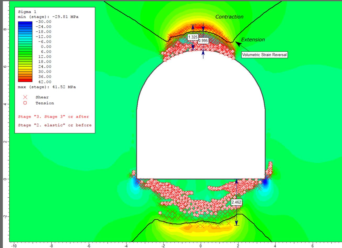
**Example of DISL application in severe rockburst environment with indications of Yielding zone and Volumetric Strain Reversal (referable to Depth of Failure of Martin et al., 1999).**
