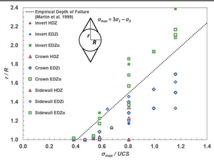
← In situ-measurements of EDZ depths compared with Martin et al. equation for DoF.
