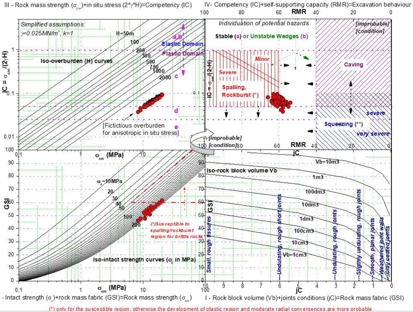
The same classification for spalling depth is applied in the GDE multiple graph
