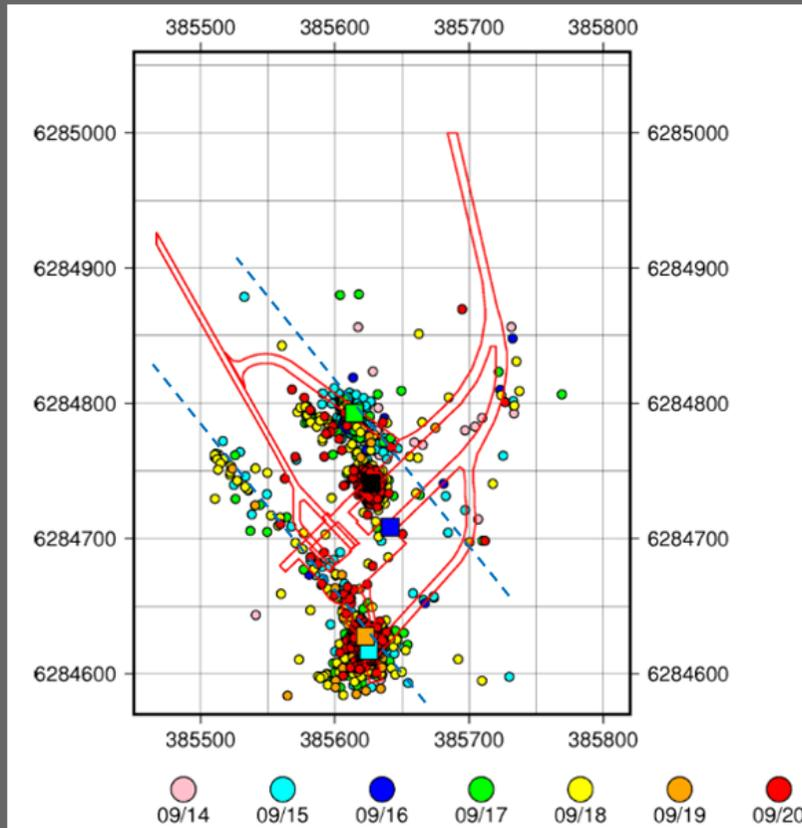
Example of seismic monitoring weekly report for tunnels of Hydroelectric project in Andean region showing the concentration of events ( $M_w = -3 \div 1$ )
