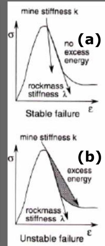
The lower the **LSS** is or the softer the mine stiffness is, the higher is the energy input from the surrounding rock mass and then the Deformation Potential (**DP**)
