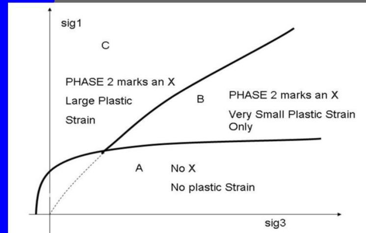
**Example of DISL application with distinction of damaged and yielding zone as a function of Maximum Shear Strain (PHASE 2=Rs2 Rocscience)**
