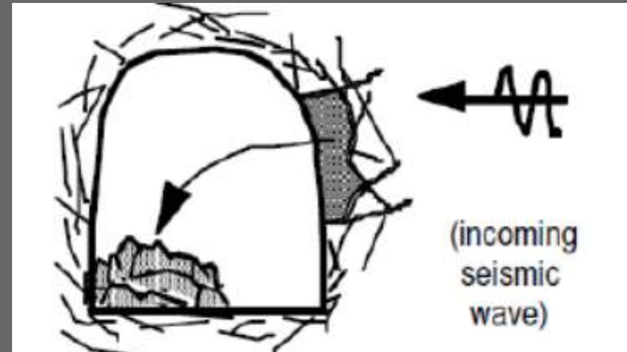
Example of severe event with failure of support in andesitic rock. Probably combined 1-2 mechanism (Estimated released Energy 25-30kJ/m<sup>2</sup>)
