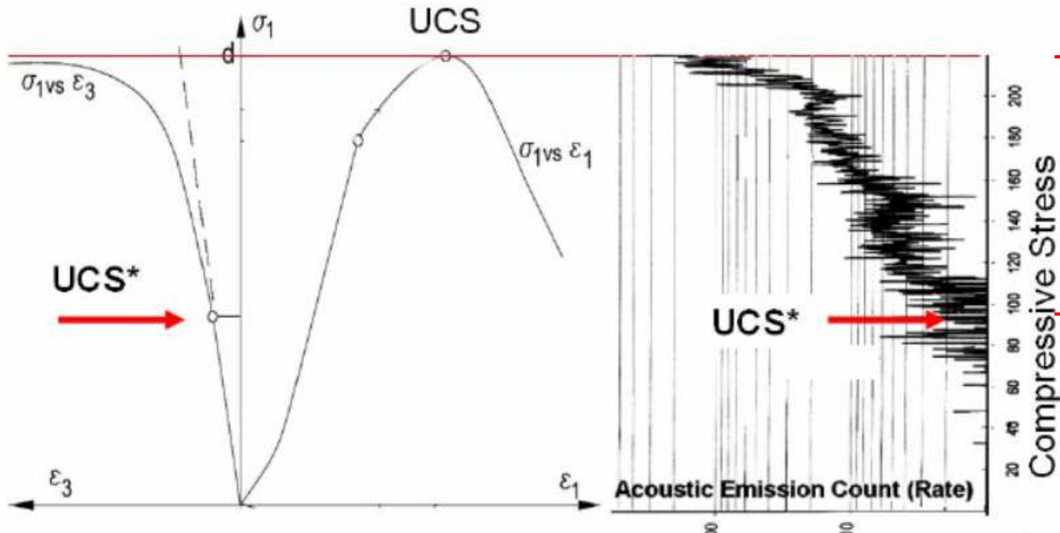
The higher the difference, the higher the stored energy and then the potential for violent failure
