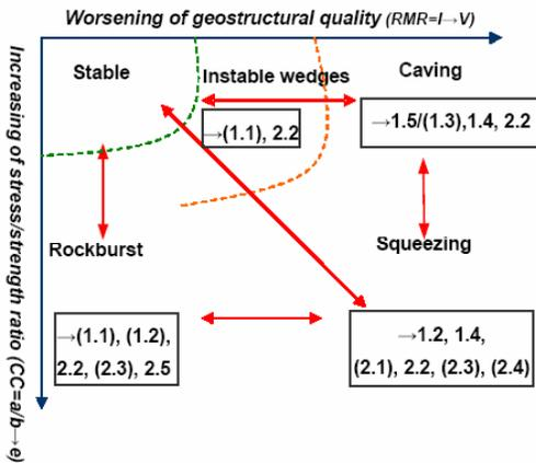
Fig.2.2: Conceptual scheme for a general setting of the ground behaviour upon excavation. The numbers in the box refer to the attempt of association of stabilisation measures later described in section 2.2. (..),/=eventual, alternative measure
