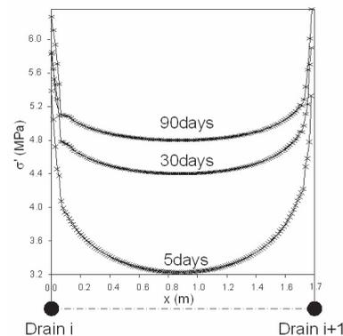
Figure 5 - Isochrones of the isotropic effective stress at 5, 30, 90 days along the line joining two drains
