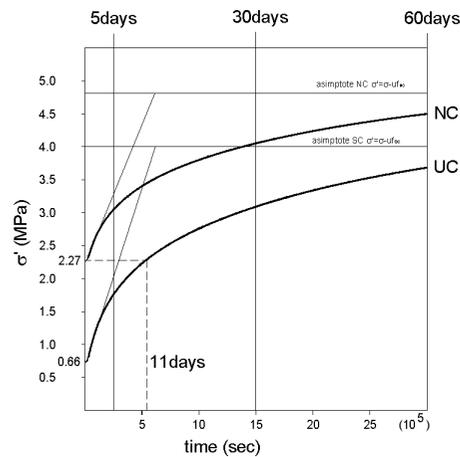
Figure 6 - Evolution with time of isotropic effective stress at the center of the line joining two drains respectively for NC and UC
