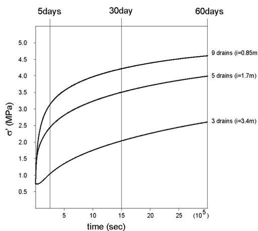
Figure 7 - Trend with time of the isotropic effective stress at a location 30cm far from a drain respectively for 3, 5, 9 drains per quarter.
