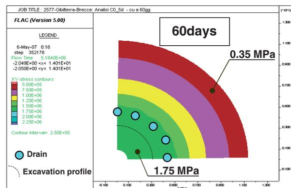
Figure 8 - Patterns at 5, 30, 60 days of  $c_u$  for 5 drains per quarter
