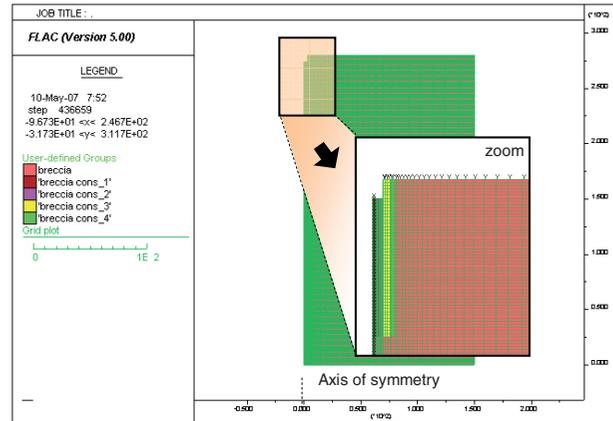
Figure 3 - Axial-symmetrical FLAC model
