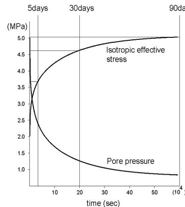
Figure 4 - Evolution of pore pressure and isotropic effective stress in a location 30cm far from a drain
