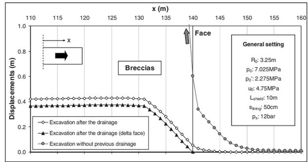
Figure 11 - Axial-symmetrical model: longitudinal profile of radial displacement
